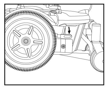
Figure 9. Freewheel Mode (Drive Disengaged)
